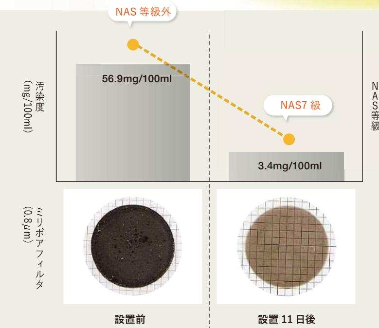
The graph illustrates the effectiveness of the ROT filter. The Y-axis represents '汚染度 (mg/100ml)' and the X-axis represents 'NAS等級'. A dashed line shows the oil contamination level decreasing from 56.9 mg/100ml (NAS grade 7) to 3.4 mg/100ml (NAS grade 7). Below the graph, two circular images show the 'ミリボアフィルタ' (rotor filter) before and after installation.
